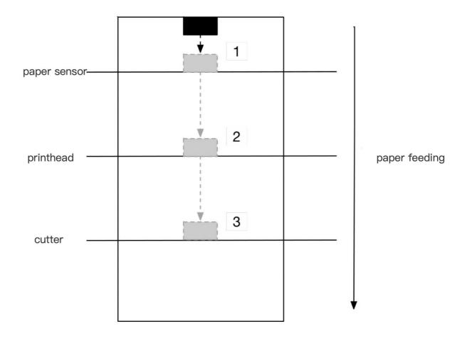
In black mark printing mode, if the sensor detects that there is no paper, it will automatically feed paper 7mm. If still no paper is detected, the printer will process it as no paper; and if paper is detected after that, the printer will process it as a black mark.
