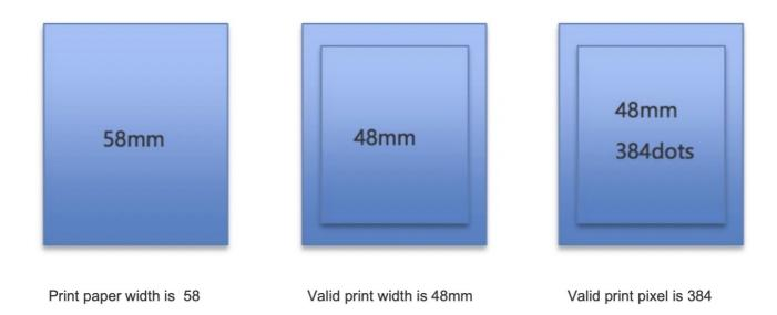
Note: SUNMI printers support the print paper of 58mm and 80mm width. This document takes the 58mm print paper as an example to illustrate the printer's supported parameters. 80mm paper has similar specifications.
