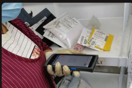
Parcel collection and sorting, OCR-based data capture, SUNMI Smart Mobile Terminals, Cainiao, China.
